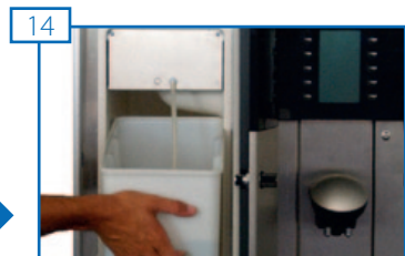
Replace milk container and close door. PRESS CLEAN.
