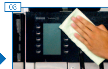
08 Clean the Evolution Plus and optional accessories with a damp microfiber cloth.
