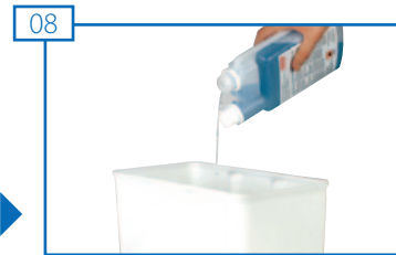
Pour 60 ml of the liquid cleaner and 1 liter of water into the milk container.
