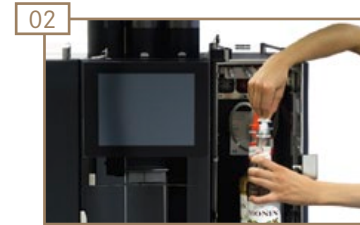
02 Place syrups in the Flavour Station and insert all hoses.
